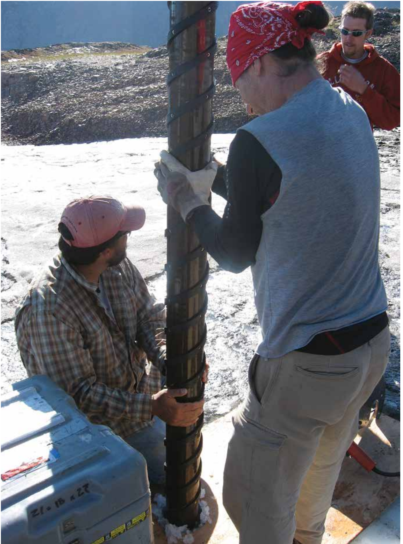
Craig Lee (left) and his colleagues Jay Kyne (facing Lee) and Ben Woods start to drill into an ice core. This is the only invasive technique the researchers employ.
